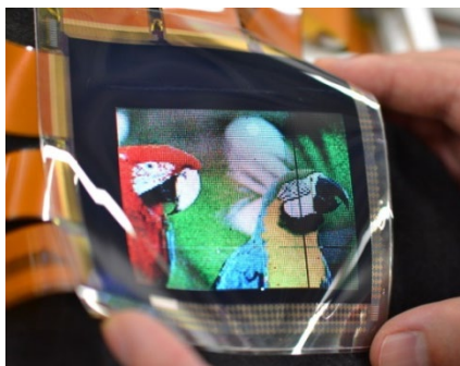
Flexible color OLED driven by OTFTs
